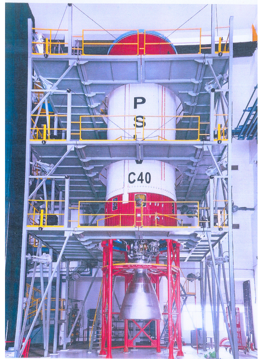
Fig.3 PSLV Second Stage with Vikas Engine at the Bottom (Courtesy : ISRO)
